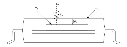
Notes: 5.  $heta_{J\!A}$  should be confirmed with what heat sink thermal resistance. If no heat sink contacting,  $heta_{J\!A}$  is almost the same as  $heta_{J\!C}$  .
