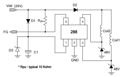
Notes: 4. The optional Capacitor C1 and Diode D3 are for power stabilization. C1 is recommended to be E-Cap., luF/25V; D3 is recommended to be Zener Diode, Vz =27V. Which C1 and D3 value need to be fine tuned to optimize design for different coils and power suppliers.
